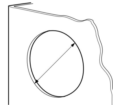
Make the mounting hole as follows. The mounting hole cut dimensions is 50 mm (2 in.)
